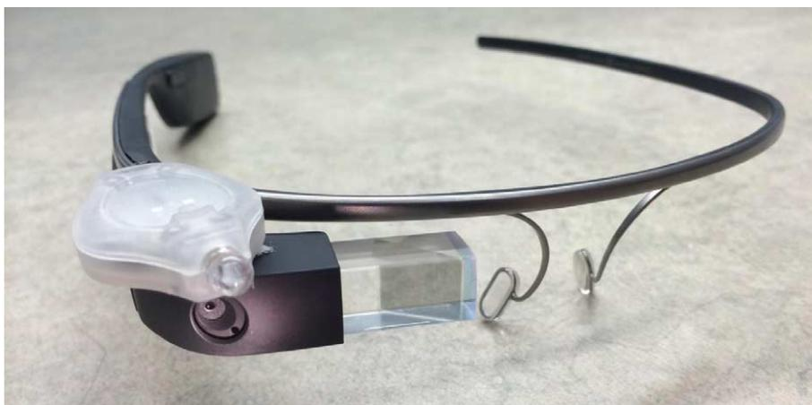
**Figure 1:** Google Glass with LED lighting apparatus fixed directly superior to aperture. During use, tissue paper is placed in front of the light for diffusion.
