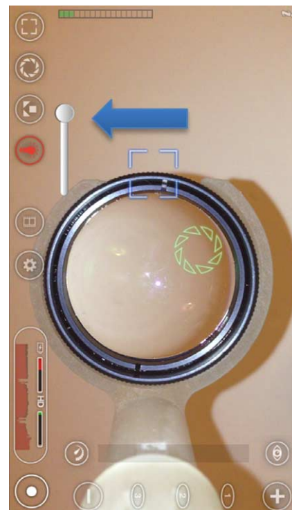
Figure 2e: Screenshot of adapter and condensing lens in place as imaged through the FilmicPro application with constant flash on lowest intensity indicated by the blue arrow
