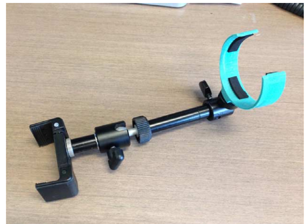
Figure 1a: Mechanical prototype of lens-to-smartphone mount with 3D printed Panretinal 2.2 condensing lens holder
