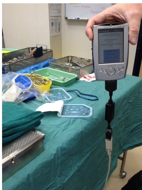
Figure 3: Cable connection between the Dell Axim X5 to the programming wand
