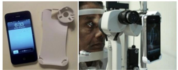
**Figure 2.** The smartphone slit-lamp adaptor. Image courtesy of eyewiki.aa.org
